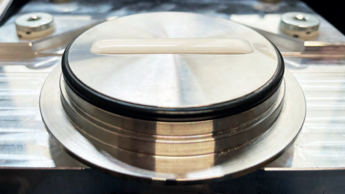
Milk on the surface of an ATR sensor. In the future, sensors like this should eliminate the need for time-consuming laboratory measurements.
