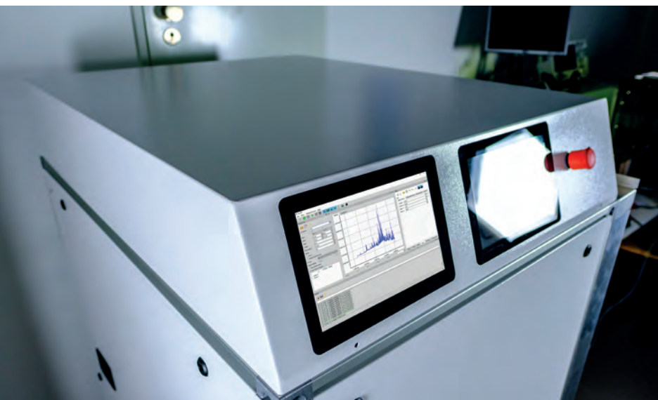
The LIBS measurement system, here in a laboratory at Fraunhofer ISIT, provides information about the chemical composition of electrode foil.
